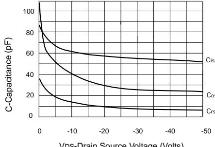
**Capacitance v drain-source voltage**
