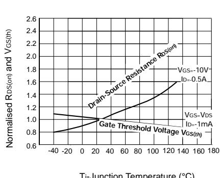
**Normalised  $R_{DS(on)}$  and  $V_{GS(th)}$  vs Temperature**
