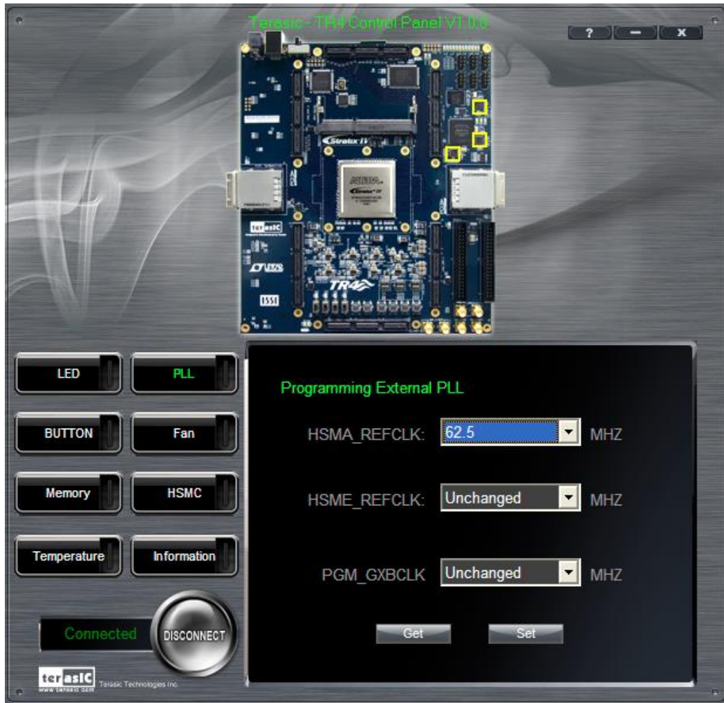
Figure 3-10 Programmable External PLL Configured through Control Panel
