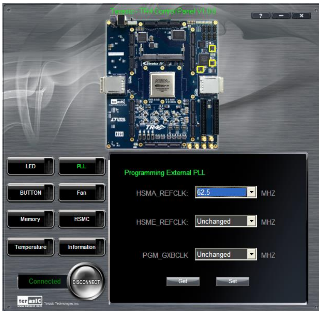
Figure 3-10 Programmable External PLL Configured through Control Panel
