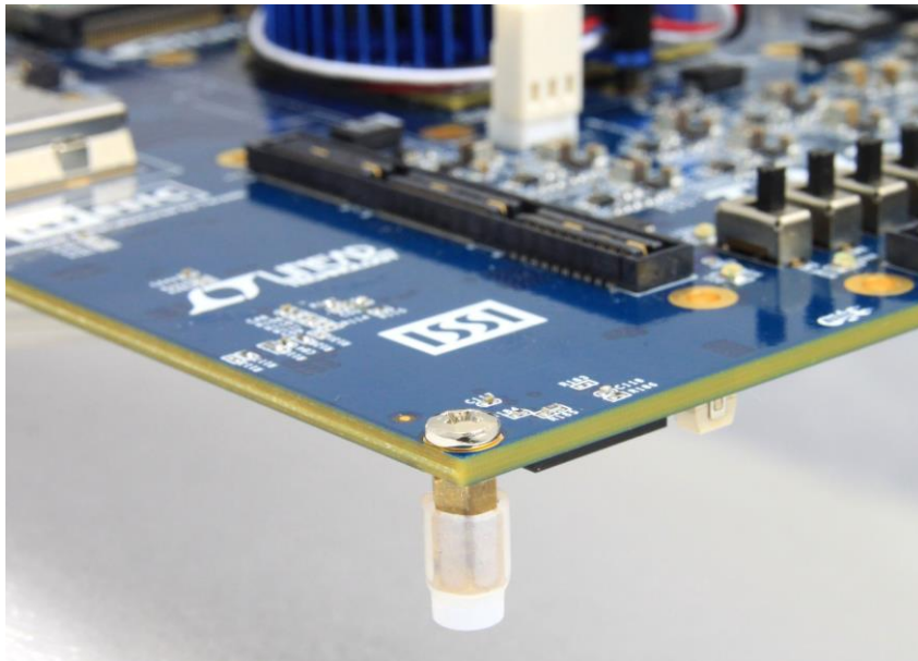
Figure 1-4 Mount Silicon Foot Stands
