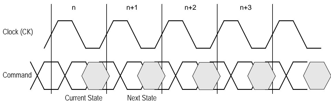
**Current State and Next State Definition for: Pipelined and Flow Through Read Write Control State Diagram**
