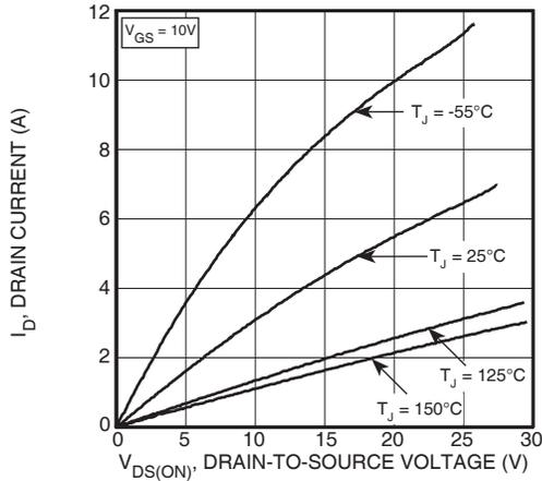
Figure 1, Output Characteristics
