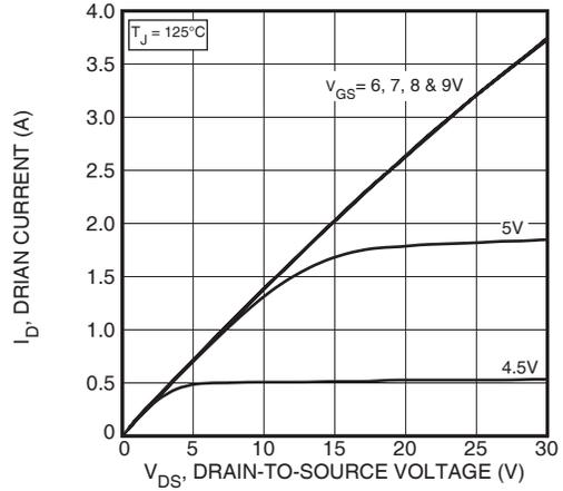
Figure 2, Output Characteristics
