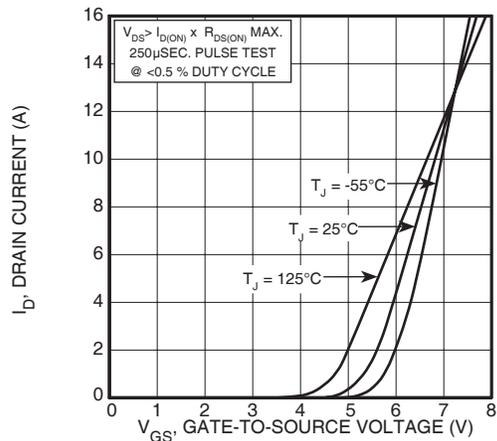
Figure 4, Transfer Characteristics
