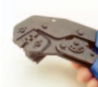
1. Cycle the CCT - SLE / SLC hand tool to the open position.
