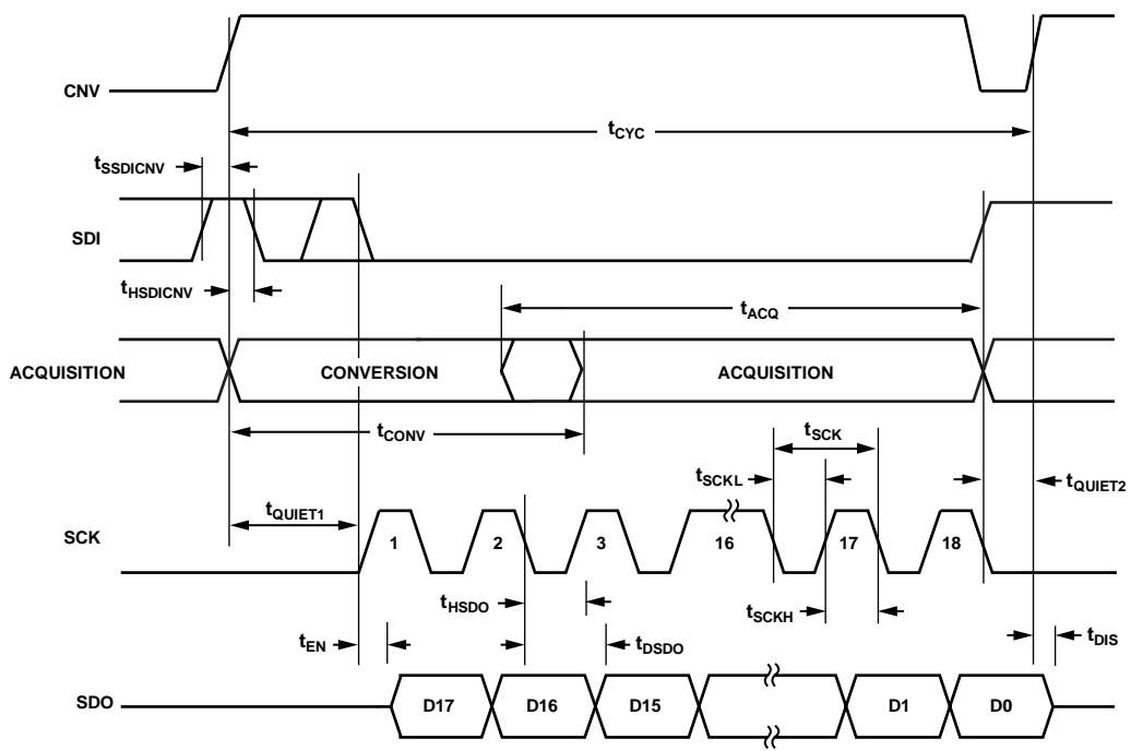
Figure 61. CS Mode, 4-Wire Turbo Mode Timing Diagram
