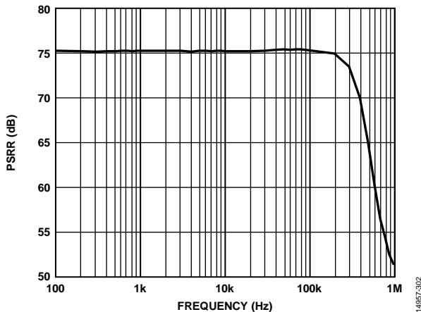
Figure 48. PSRR vs. Frequency,  $V_{DD} = 1.8\text{ V}$ ,  $V_{IO} = 3.3\text{ V}$ ,  $V_{REF} = 5\text{ V}$ ,  $25^\circ\text{C}$
