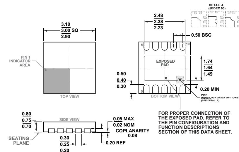
Figure 71. 10-Lead Lead Frame Chip Scale Package [LFCSP]
