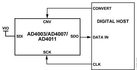
Figure 56. CS Mode, 3-Wire Without Busy Indicator Connection Diagram (SDI High)
