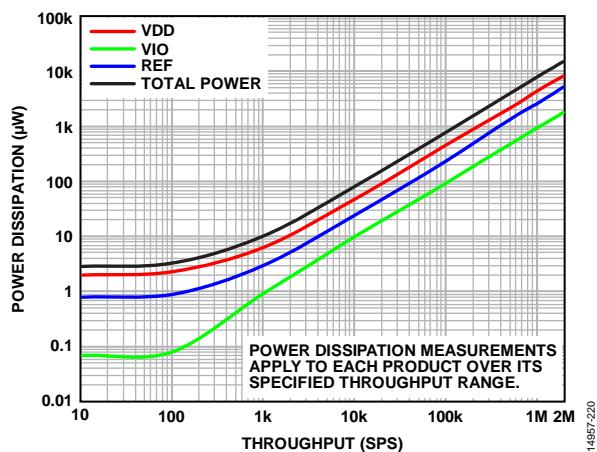
Figure 49. Power Dissipation vs. Throughput,  $V_{DD} = 1.8\text{ V}$ ,  $V_{IO} = 3.3\text{ V}$ ,  $V_{REF} = 5\text{ V}$ ,  $25^\circ\text{C}$
