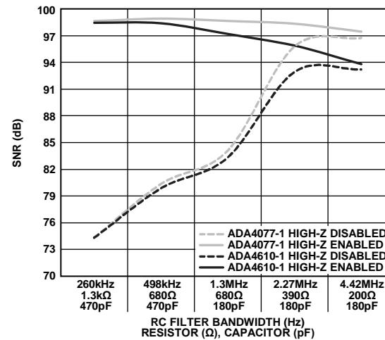
Figure 46. SNR vs. RC Filter Bandwidths for Various Precision ADC Drivers,  $f_{IN} = 1$  kHz (Turbo Mode On, High-Z Enabled/Disabled),  $V_{DD} = 1.8$  V,  $V_{IO} = 3.3$  V,  $V_{REF} = 5$  V,  $25^\circ\text{C}$
