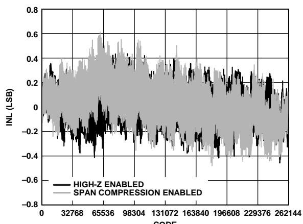
Figure 8. INL vs. Code, High-Z and Span Compression Modes Enabled,  $V_{REF} = 5\text{ V}$
