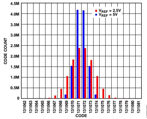
Figure 15. Histogram of a DC Input at Code Transition,  $V_{REF} = 2.5\text{ V}$  and  $V_{REF} = 5\text{ V}$
