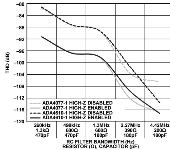
Figure 47. THD vs. RC Filter Bandwidths for Various Precision ADC Drivers,  $f_{IN} = 1$  kHz (Turbo Mode On, High-Z Enabled/Disabled)  $V_{DD} = 1.8$  V,  $V_{IO} = 3.3$  V,  $V_{REF} = 5$  V,  $25^\circ\text{C}$
