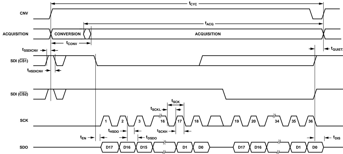
Figure 63. CS Mode, 4-Wire Without Busy Indicator Serial Interface Timing Diagram
