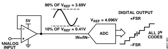
Figure 43. Span Compression
