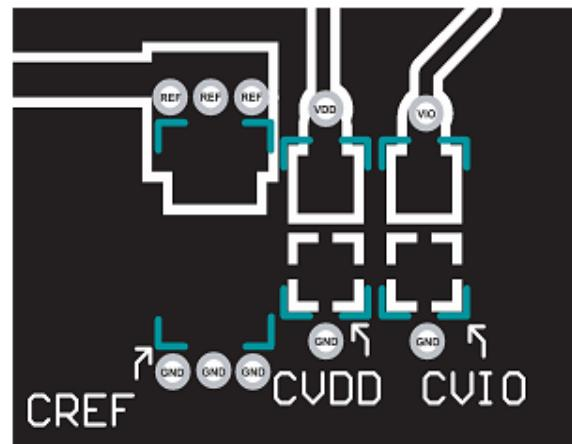
Figure 69. Example Layout of the AD4003 (Bottom Layer)
