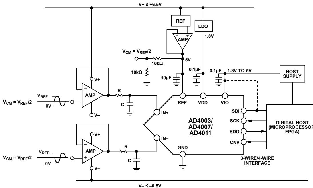
*Figure 34. Typical Application Diagram with Multiple Supplies*
