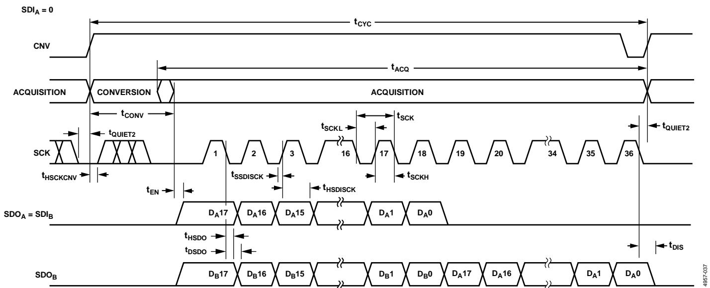
Figure 67. Daisy-Chain Mode Serial Interface Timing Diagram
