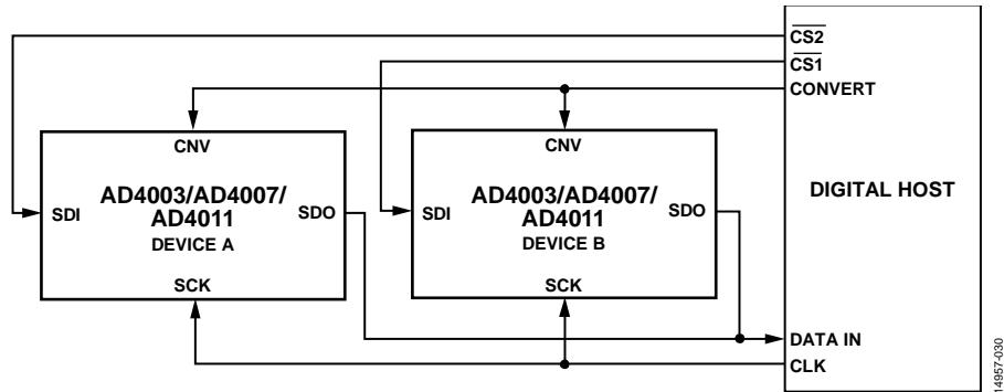
Figure 62. CS Mode, 4-Wire Without Busy Indicator Connection Diagram
