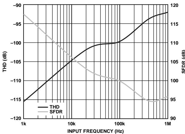
Figure 41. THD and SFDR vs. Input Frequency,  $VDD = 1.8\text{ V}$ ,  $VIO = 3.3\text{ V}$ ,  $VREF = 5\text{ V}$ ,  $25^\circ\text{C}$
