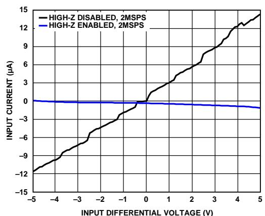
Figure 2. Input Current vs. Input Differential Voltage
