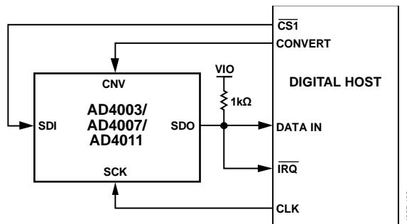
Figure 60. CS Mode, 4-Wire Turbo Mode Connection Diagram
