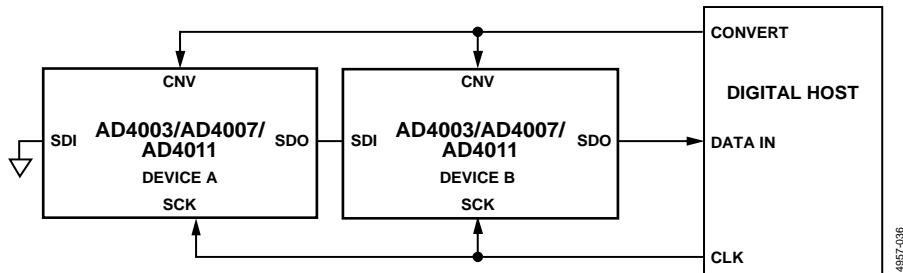
Figure 66. Daisy-Chain Mode Connection Diagram
