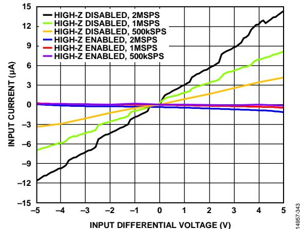
Figure 44. Input Current vs. Input Differential Voltage,  $VDD = 1.8\text{ V}$ ,  $VIO = 3.3\text{ V}$ ,  $V_{REF} = 5\text{ V}$ ,  $25^\circ\text{C}$
