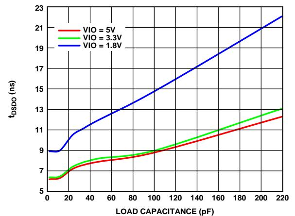
Figure 31. t<sub>DSDO</sub> vs. Load Capacitance
