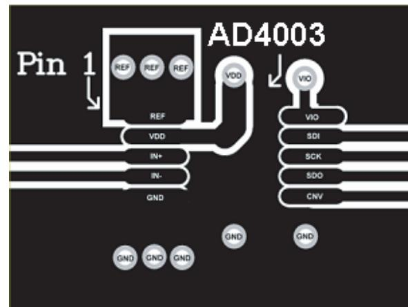
Figure 68. Example Layout of the AD4003 (Top Layer)
