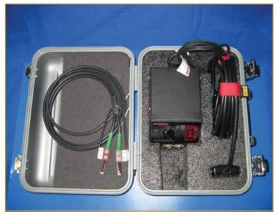
RH-396X Tinel-Lock Installation Tool
