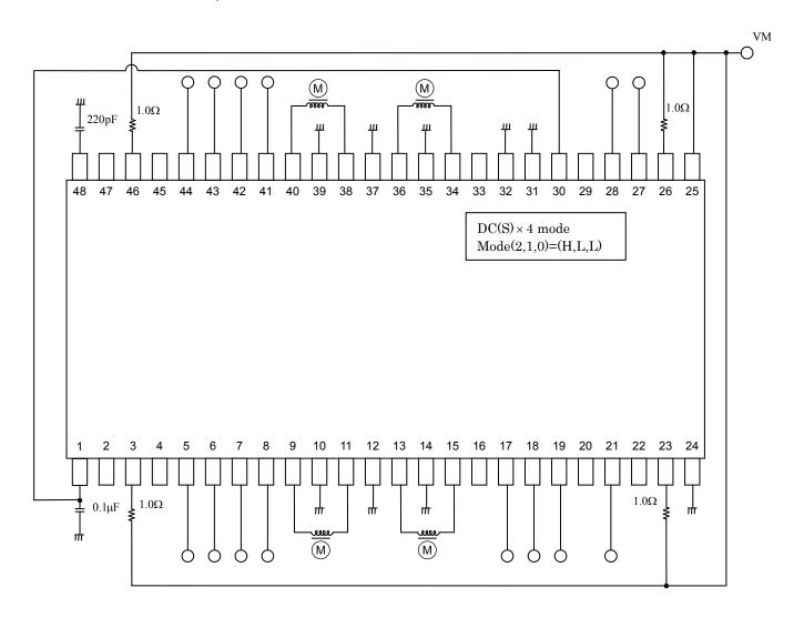
Note: Adding bypass capacitor is recommended if necessary.
