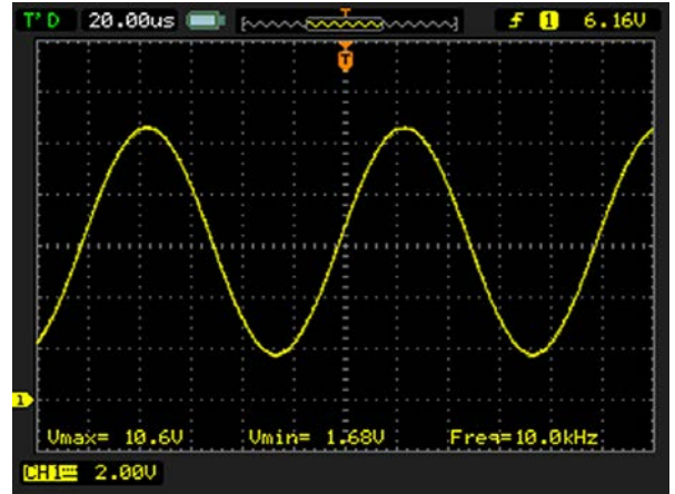
Figure 7. Signal at the Resolver Input When Using High Performance Mode
