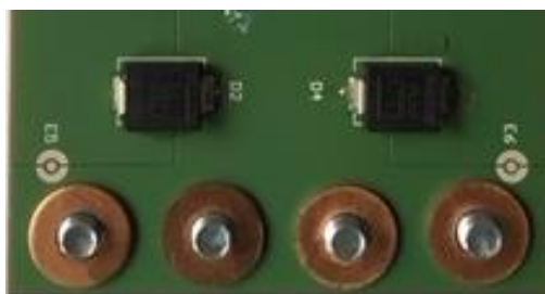
Figure 6 Copper washers between PCB and bus bar
