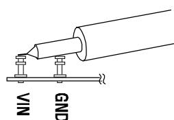
Figure 2. Measuring Input or Output Ripple
