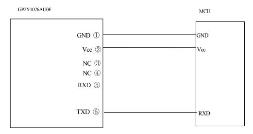
\*) Without connecting about a RXD terminal for a sensor, please use as an OPEN terminal.
