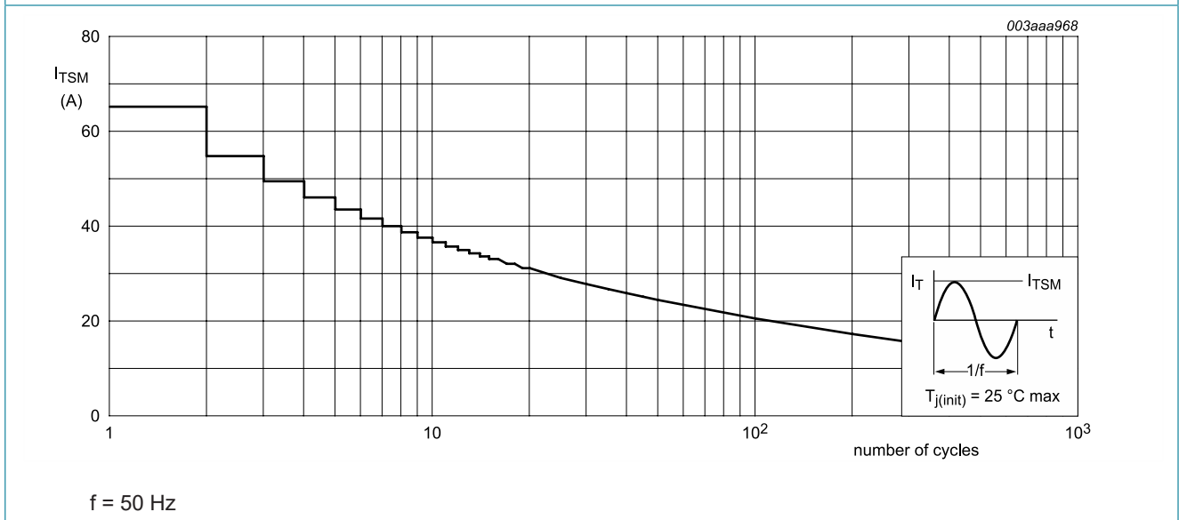
Fig. 4. Non-repetitive peak on-state current as a function of the number of sinusoidal current cycles; maximum values
