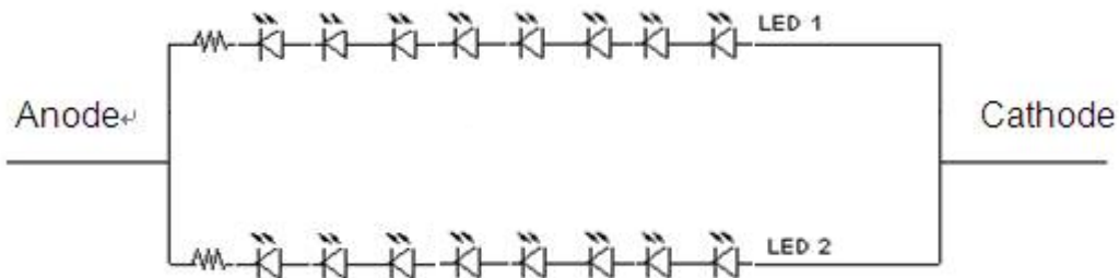
Figure 5 LED Light Bar Structure
