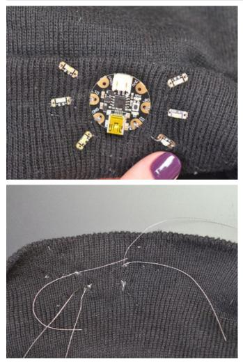
Next hook up the + connections from each of GEMMA's outputs to three pixels. We stitched from one sequin to the GEMMA, then over to another sequin and on to the third sequin before going back to the first, making a sort of square that results in the thread tails being in the same place.
