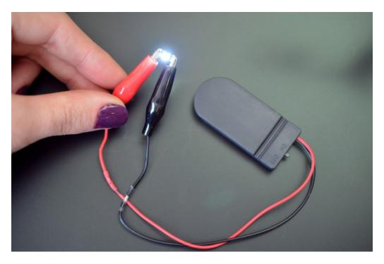
Simply connect 3 to 6VDC to the + pin and ground to the - pin, and the LED on the board will light up. In the photo above we've soldered alligator clips to a 2x2032 coincell battery holder (~6V). You could also use a single CR2032 sewable coincell holder-- you do not need a microcontroller to drive these sequins, unless you want them to blink or fade.
