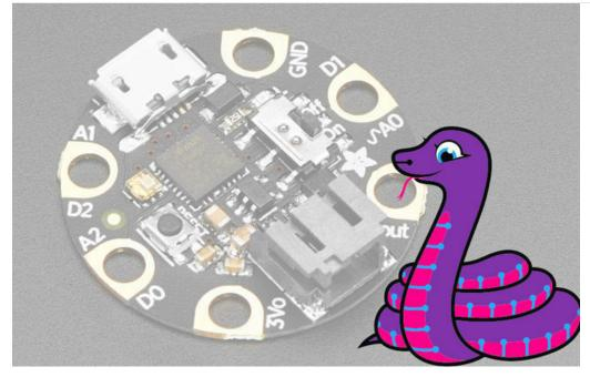
**GEMMA MO** boards can run **CircuitPython** — a different approach to programming compared to Arduino sketches. In fact, **CircuitPython comes factory pre-loaded on GEMMA MO**. If you've overwritten it with an Arduino sketch, or just want to learn the basics of setting up and using CircuitPython, this is explained in the **Adafruit GEMMA MO** guide (https://adafru.it/z1B).
