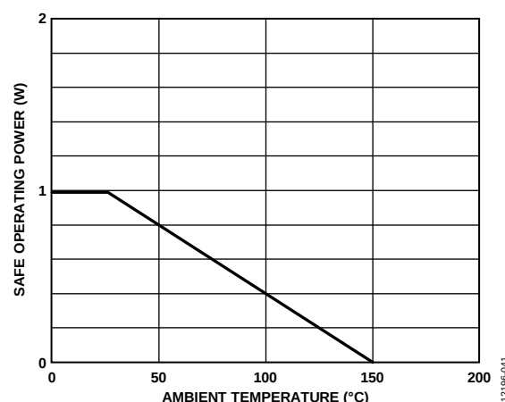
Figure 4. AD7403-8 Thermal Derating Curve, Dependence of Safety Limiting Values with Case Temperature per DIN V VDE V 0884-10
