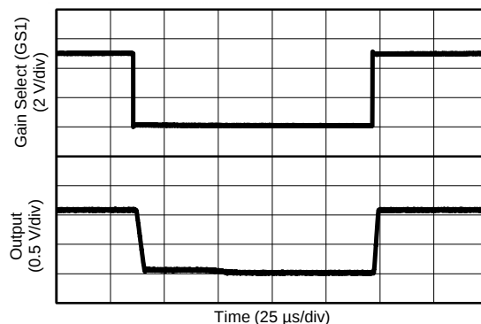
Figure 28. Gain Change Output Response (Gain = 50 V/V to 200 V/V)
