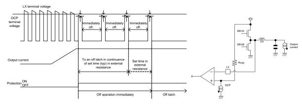
**Figure.6 Overcurrent protection**
