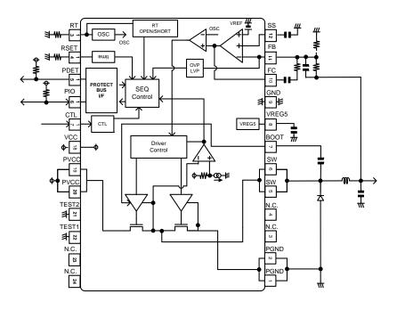
Figure.2 Block diagram, Application diagram
