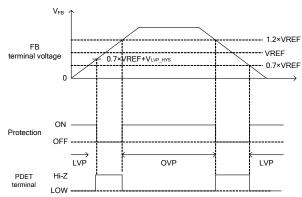
Figure.5 Low voltage / overvoltage protection
