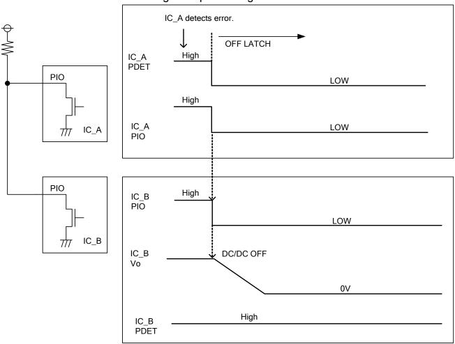
When two or more BD8628EFV/BD8624FV is used at the same time, If one IC error detects, all IC becomes DC/DC OFF at the same time.
