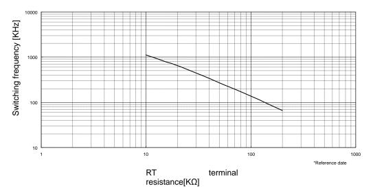
Figure.4 Terminal RT resistance-oscillation frequency
