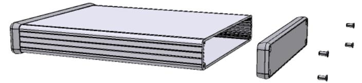
EXTRUSION DESIGNED FOR 160MM WIDE PC BOARD
