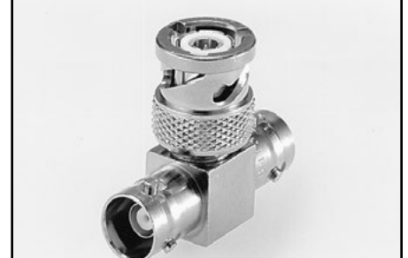
Model 237-TRX-T: 3-slot male to dual 3-lug female triax tee adapter for use with 7078-TRX cables and 7072/7072-HV Semiconductor Matrix Cards. High voltage rating for use with Model 6517B Electrometer.
