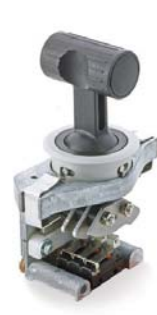
Lever switch, 2-5 positions, plug-in or screw terminals, aluminium bezel, silver contacts with positive opening, 33.5mm mounting
