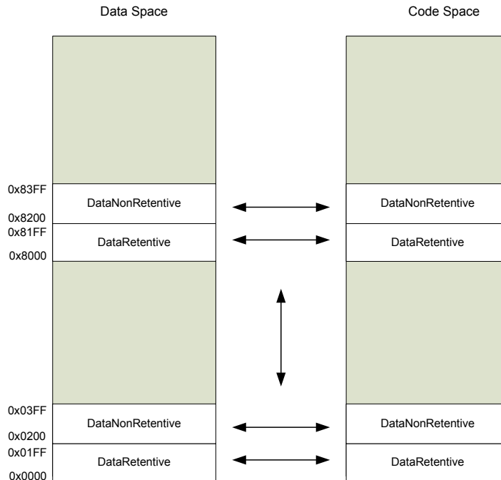
Figure 37. Configurability of SRAM address space location
