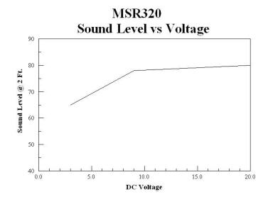
For audible alarm model MSR320R, the sound level will vary from 65 dB at 2 ft. at 3 Vdc up to 80 dB at 2 ft. at 20 Vdc. By varying the voltage from 3 to 20 Vdc, the sound level can be varied by 15 dB. A 10 dB drop in sound level will make the alarm sound half as loud.
