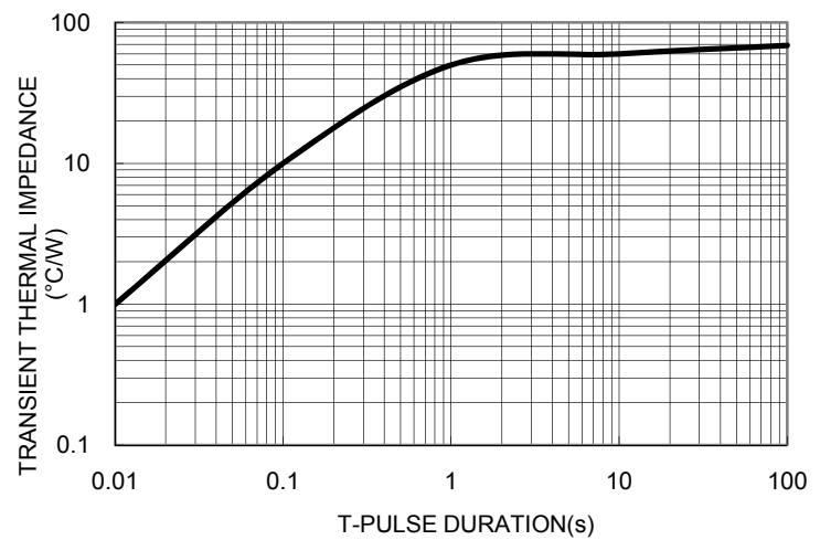
FIG. 6 TYPICAL TRANSIENT THERMAL IMPEDANCE PER LEG
