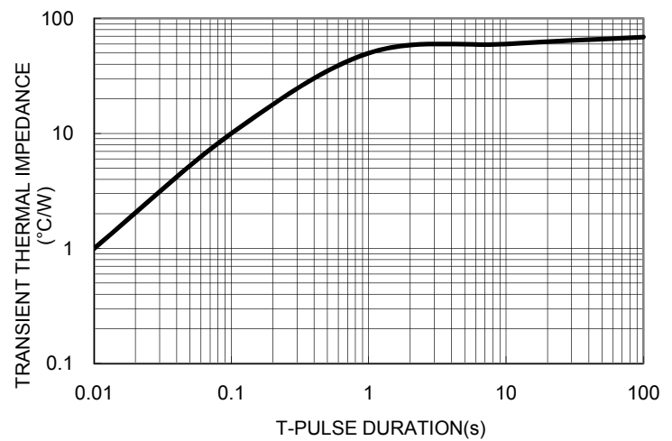
FIG. 6 TYPICAL TRANSIENT THERMAL IMPEDANCE PER LEG
