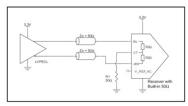
Figure 1C. IN/nIN Input with Built-In 50Ω Driven by an LVPECL Driver
