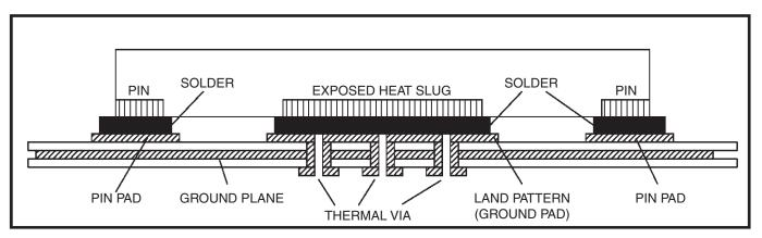
Figure 3. P.C. Assembly for Exposed Pad Thermal Release Path – Side View (drawing not to scale)
