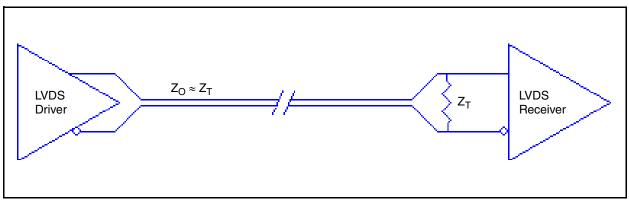
Figure2A. Standard LVDS Termination
