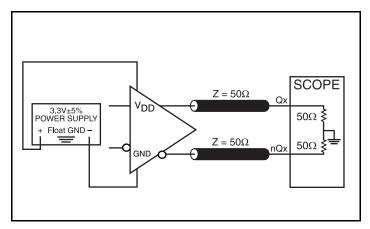
**LVDS Output Load AC Test Circuit**
