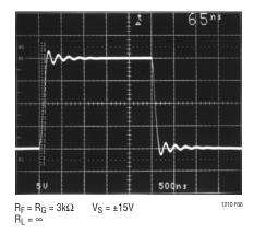
Figure 6. Large-Signal Response,  $C_1 = 10,000pF$
