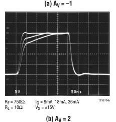
Figure 4. Large-Signal Response vs I<sub>0</sub>
