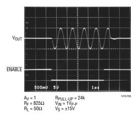
Figure 3. Shutdown Operation
