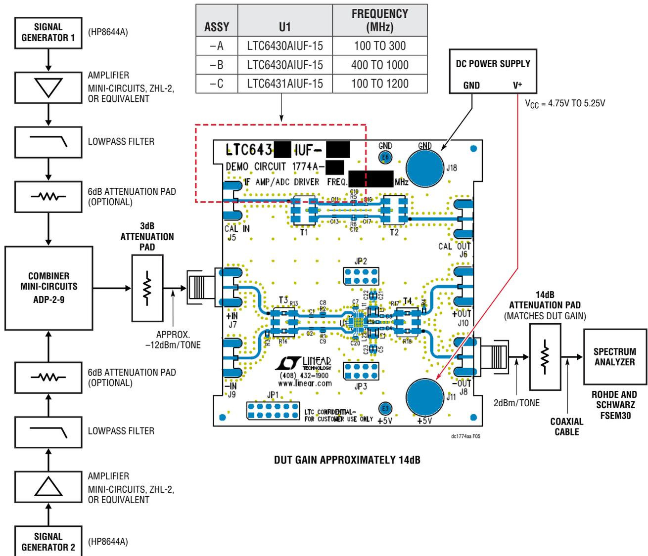
Figure 5. Proper Equipment Setup for IP3 Measurement
