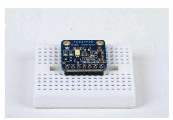
Position the Breakout Place the breakout over the exposed short end of the header pins.
