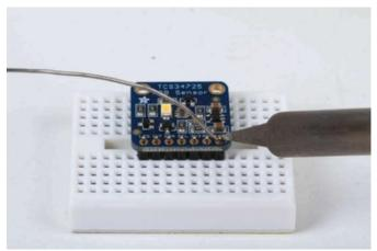
And Solder! Solder all pins to ensure good electrical contact.
