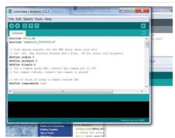
Load ColorView on the Arduino Open the ColorView example sketch and upload it to your Arduino.
