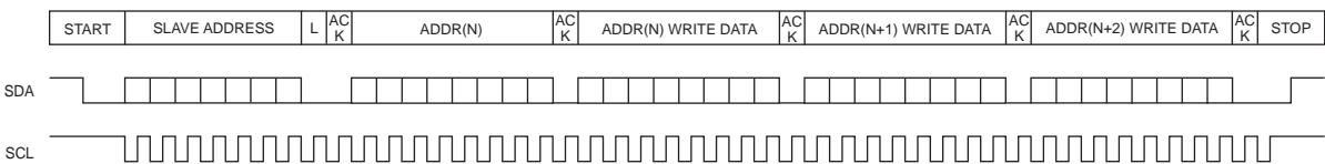
Reading format (Sequential Reading is possible)
