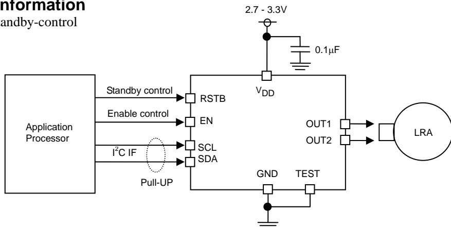
Note) When SDA&SCL signal voltages are different from VDD, even if the RSTB pin is set to Low, the IO leak current flows.
