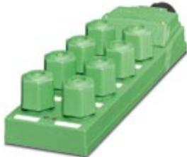
Sensor/actuator box, Connection method: QUICKON, 0.34 mm<sup>2</sup> ... 0.75 mm<sup>2</sup>, Number of slots: 6, Number of positions: 4, Slot assignment: Single, Status indication: Yes, npn; Master cable connection: Spring-cage conn. 180°, Shielding: No
