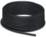
Master cable for sensor/actuator boxes, with PE conductor, unshielded, material PUR/PVC, 9-pos., 6 x 0.34 mm<sup>2</sup> and 3 x 0.75 mm<sup>2</sup>
