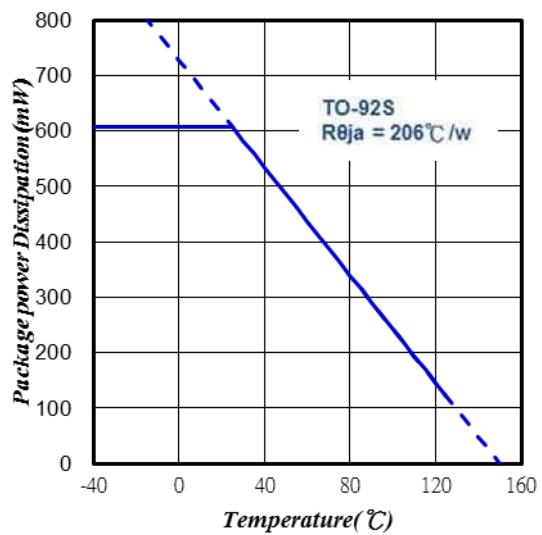
Figure 8. Temperature vs. Power Dissipation
