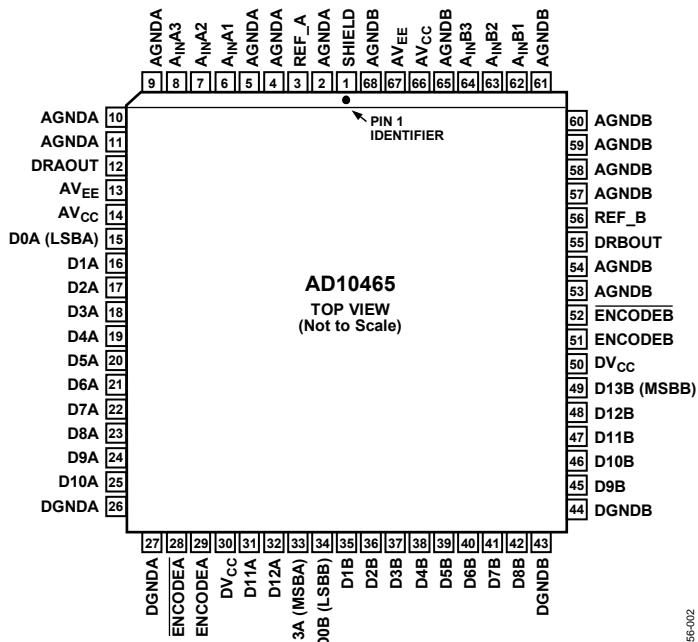
Figure 7. Pin Configuration
