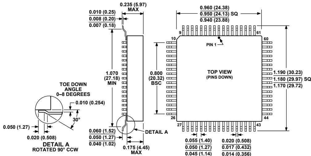
CONTROLLING DIMENSIONS ARE IN INCHES; MILLIMETER DIMENSIONS
