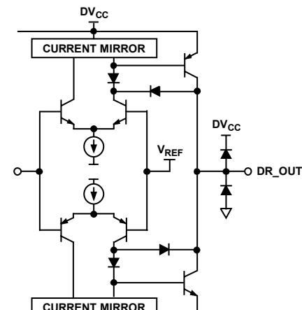
Figure 5. Digital Output Stage
