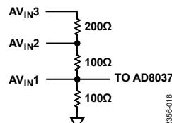
Figure 3. Analog Input Stage
