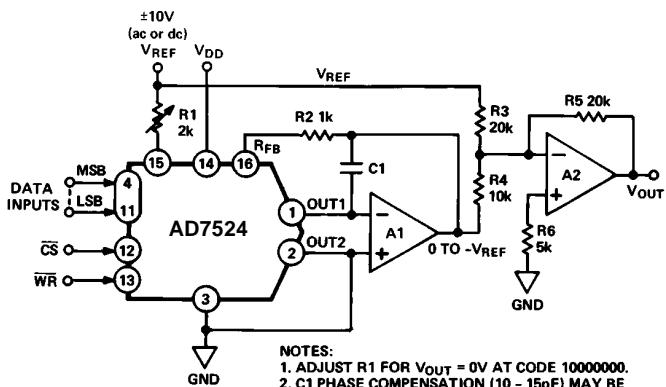
Figure 5. Bipolar (4-Quadrant) Operation
