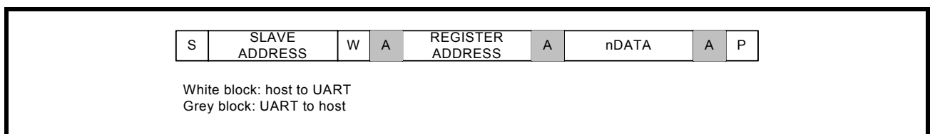
FIGURE 4. MASTER WRITES TO SLAVE (XR20M1280)
