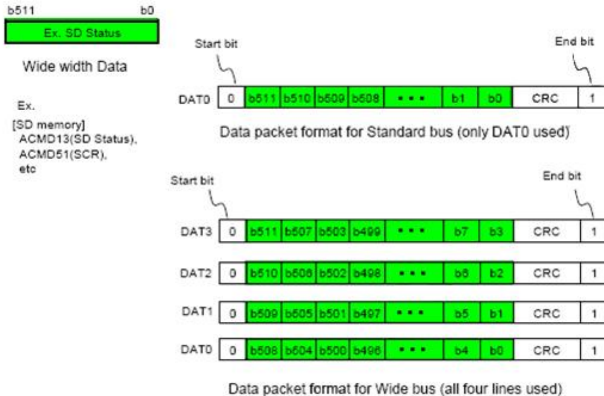
Figure 6-7: Data packet format - Wide width data
