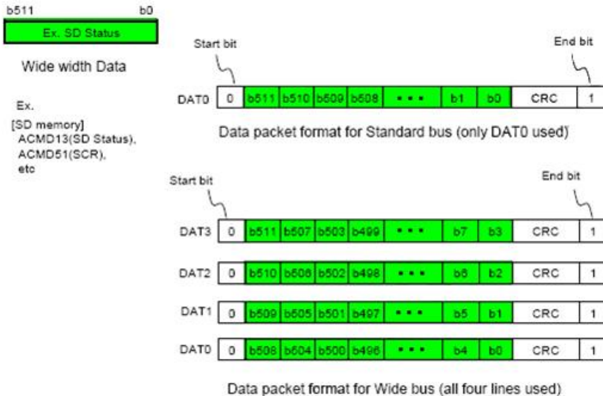
Figure 6-7: Data packet format - Wide width data
