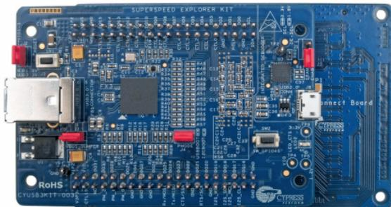
2. Plug the FMC Interconnect Board into the Xilinx<sup>®</sup> FPGA board (The Xilinx FPGA board is not part of this kit)
