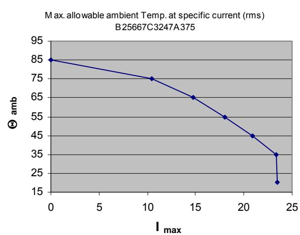
**Film capacitors – Power Factor Correction****B25667C3247A375****PhaseCap Premium Capacitors****MKK400-D-12.5-0.1****Preliminary data**
