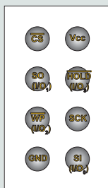
Figure 1-3. 8-ball WLCSP (Bottom View)
