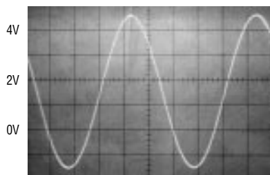
6V p-p INPUT, -1.5V TO 4.5V
