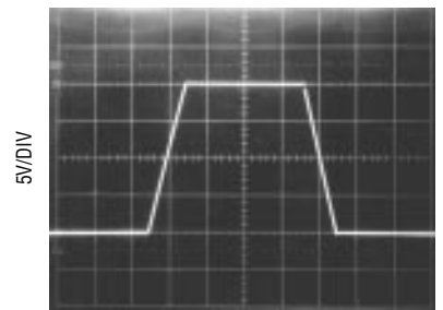
Large Signal Transient Response, VS = ±15V
