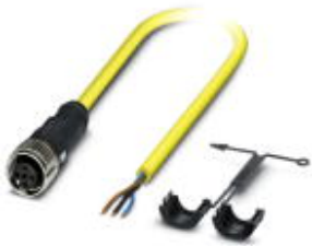
Sensor/Actuator cable, 3-position, PVC, yellow RAL 1021, free cable end, on Socket straight M12 SPEEDCON, A-coded, Cable length: 10 m
