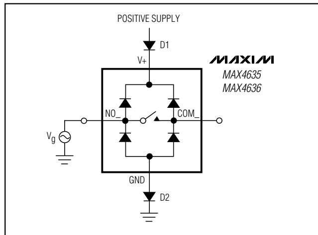
Figure 5. Overvoltage Protection Using Two External Blocking Diodes
