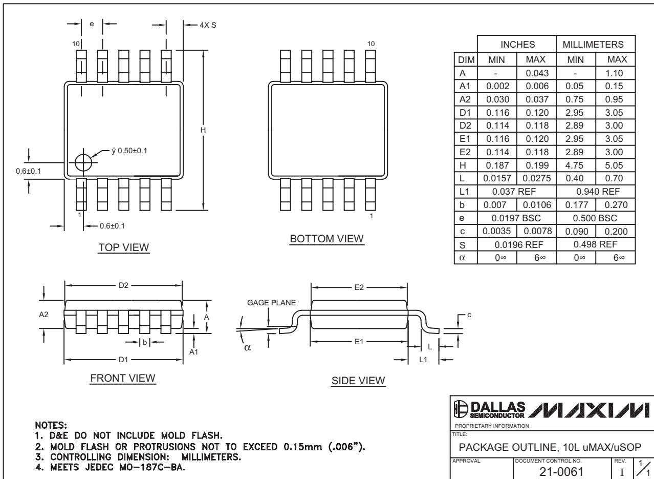
**Note:** The MAX4636 does not have an exposed pad.
