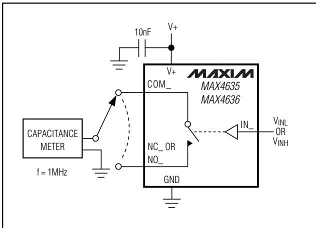
Figure 3. Channel Off/On-Capacitance
