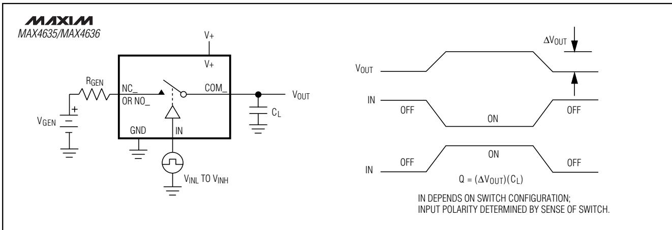
Figure 2. Charge Injection
