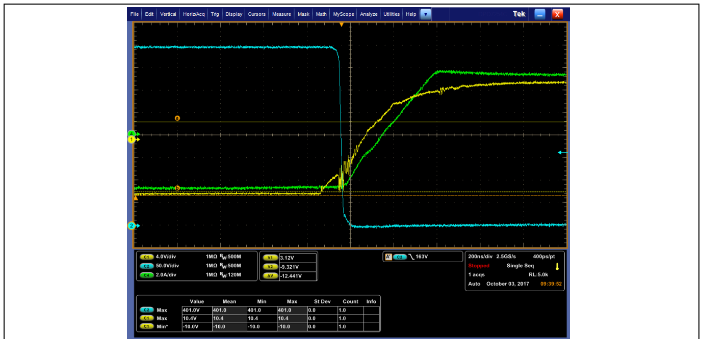
Figure 63 Leading leg achieves ZVS at 117 A. Waveforms captured on MOSFET B: V_{DS} (blue); V_{GS} (yellow); primary current (green).
