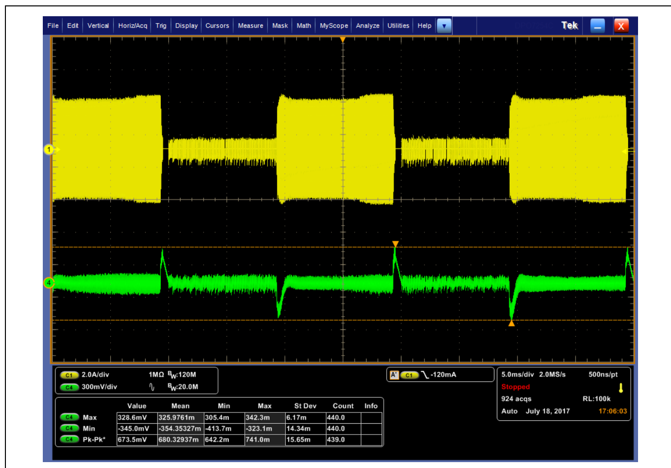
Figure 71 5 A–60 A output dynamic load. Primary current (yellow), output voltage (green).
