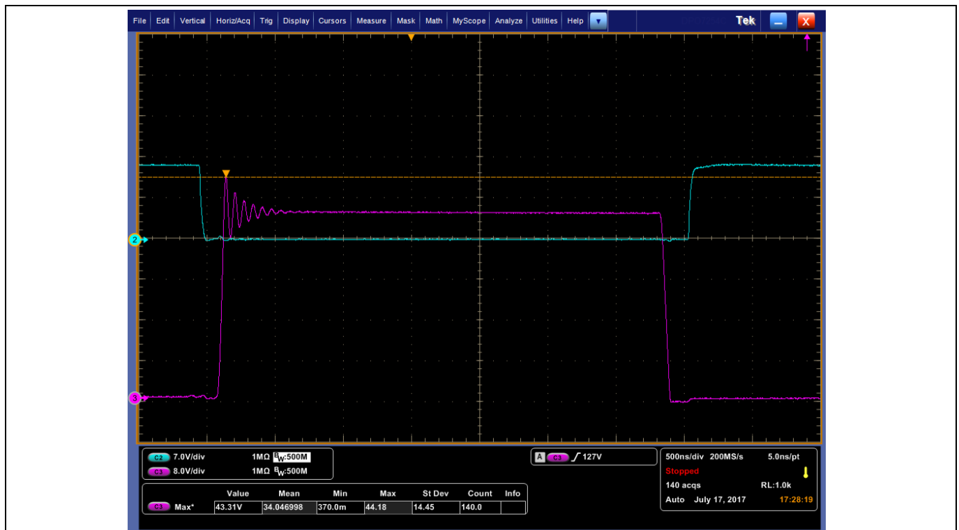
Figure 65 Synchronous turn-on/off delay at 700 W load. V_{DS} (purple) and V_{GS} (blue).
