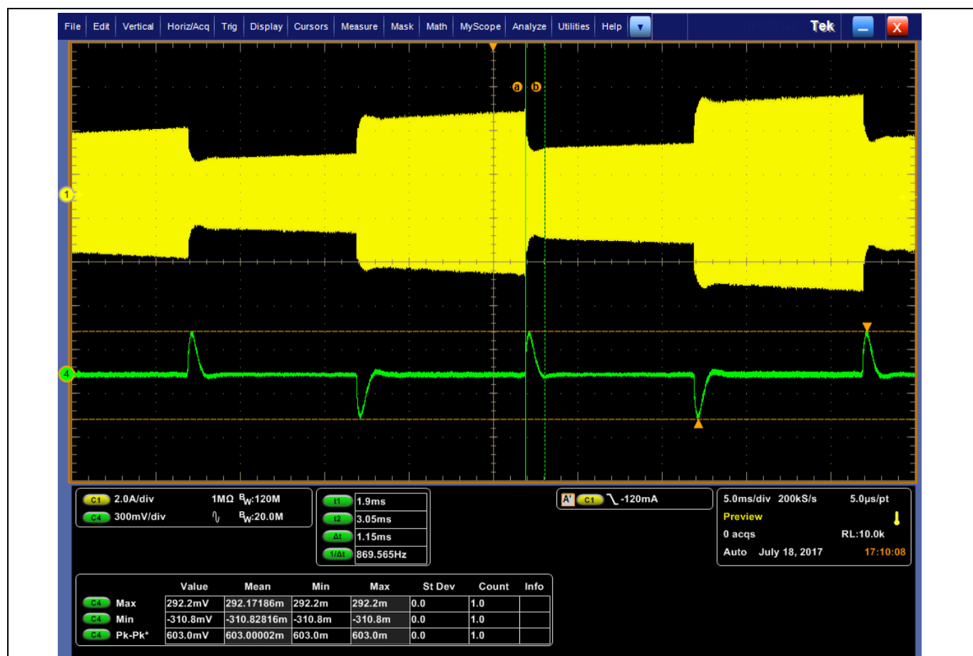
Figure 72 60 A–117 A output dynamic load. Primary current (yellow), output voltage (green).
