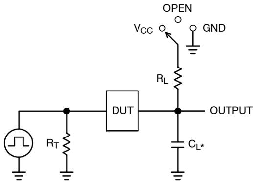
\* $C_L$  includes probe and jig capacitance
