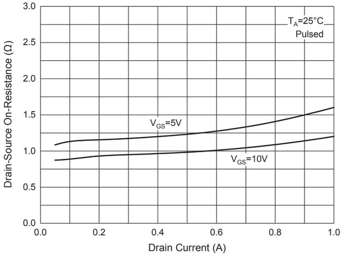
Fig. 3 -  $R_{DS(ON)} - V_{GS}$
