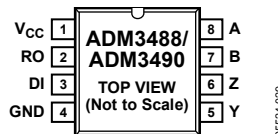
Figure 5. ADM3488/ADM3490 Pin Configuration
