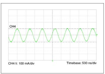
Figure 4 — Input reflected ripple current
