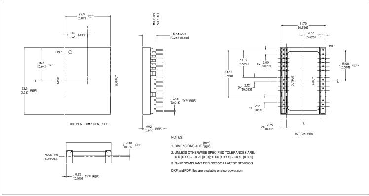
Figure 21 — PRM Through-hole mechanical outline
