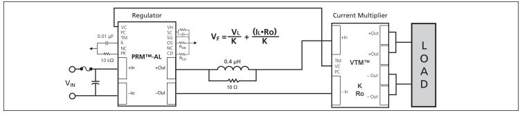
Figure 16 — Adaptive Loop compensation with output voltage trimming and soft start using the SC port.
