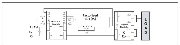
**Figure 1** — With Adaptive Loop control, the output of the VTM is regulated over the load current range with only a single interconnect between the PRM and VTM and without the need for isolation in the feedback path.
