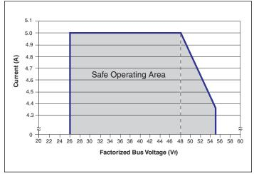
Figure 17 — P048F048T24AL rating based on Factorized Bus voltage
