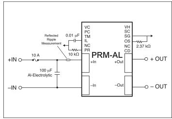
**Figure 5** — Input filter capacitor recommendation
