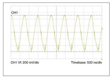
Figure 13 — Output ripple full load no bypass capacitance
