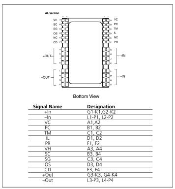
Figure 15 — PRM pin configuration
