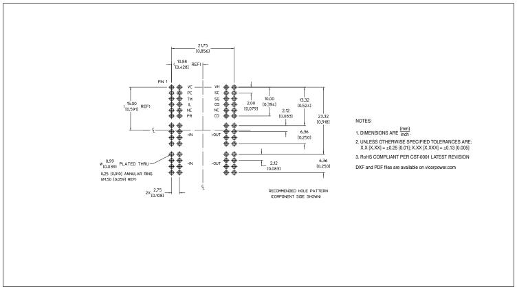
Figure 22 — PRM Through-hole PCB layout information
