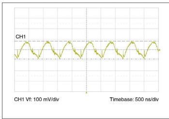
Figure 14 — Output ripple full load 10µF bypass capacitance
