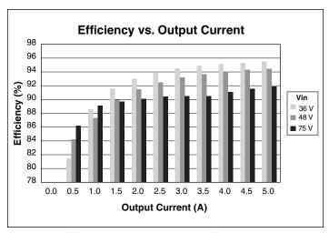
**Figure 8** — Efficiency vs. output current at 26 Vf
