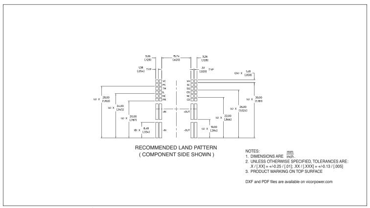
Figure 20 — PRM J-Lead PCB layout information
