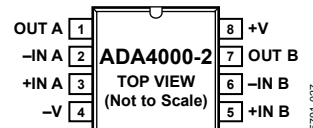
Figure 3. 8-Lead SOIC (R-8)
