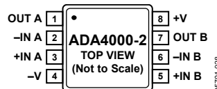
Figure 4. 8-Lead MSOP (RM-8)
